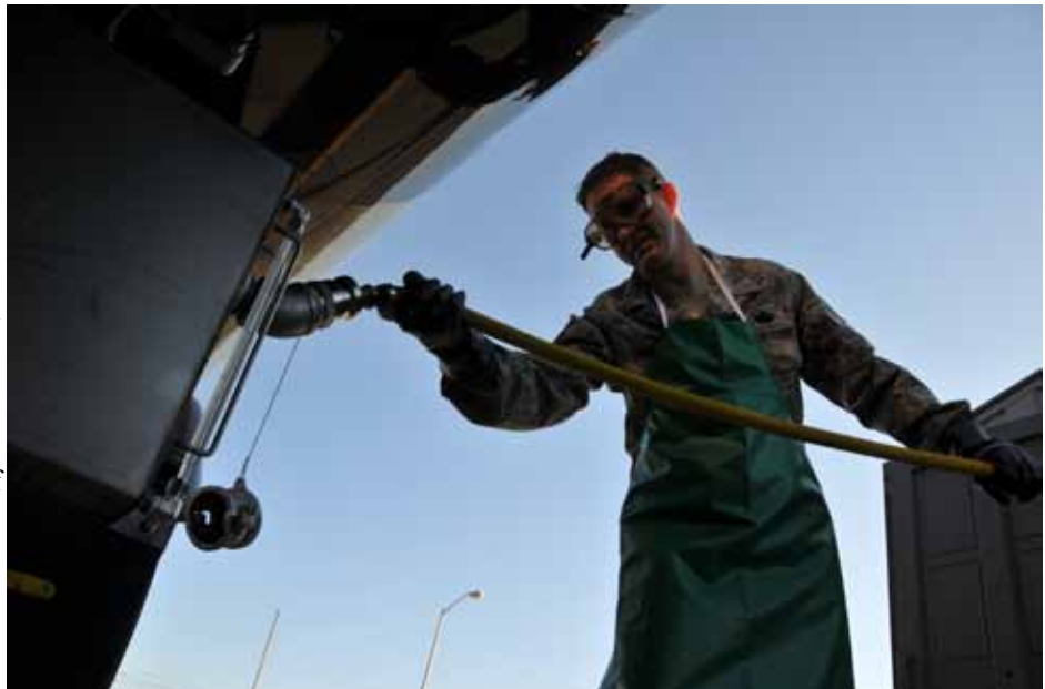
Master Sgt. William Frederick, 934th Airlift Wing fuels superintendent, pours an anti-icing additive into a fuel truck as part of the AFSSO21 "JP-8 to Jet A fuel conversion" demonstration at the Minneapolis-St. Paul Air Reserve Station, Minn. on Nov. 17. (Air Force Photo/Tech. Sgt. Jeffrey Williams)
