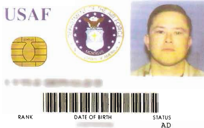
A look at the new Defense Department common access card. With a 32 kilobyte embedded computer chip, magnetic stripe and two bar codes, the "Smart Card" will eventually replace the standard military identification card. (File photo)
