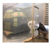
Chad Kent performs all of the ventilation surveys for the 934 AW. He already ensured the Tent Vent pulled enough air to keep TSgt Voss safe from chemicals in the paint while inside the makeshift paint booth. The Tent vent provides convenient ventilation for other processes on base that are not in fixed or predictable settings.
